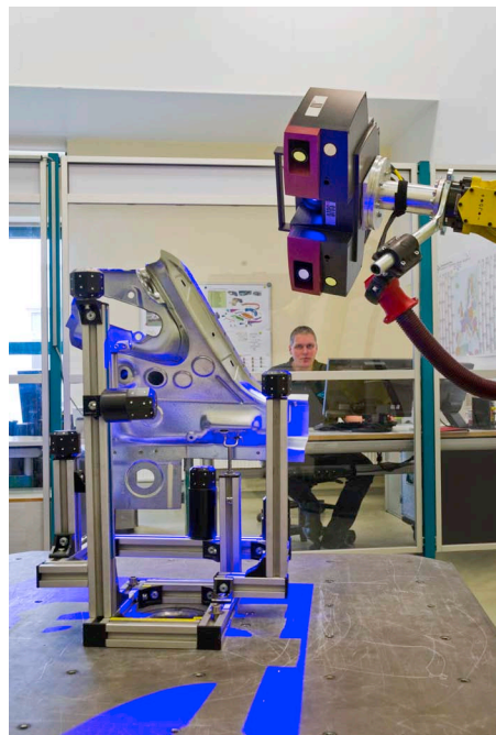
Fig. 4: The first automated solution at GEDIA: a customized measuring cell with integrated GOM equipment.
